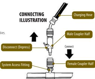
**WARNING:** Do not allow any refrigerant cylinder, connected for charging, to be exposed to system high side pressure cylinder - explosion could result!
