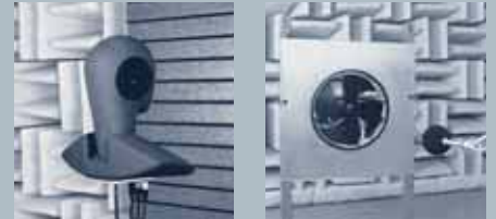
Room for precision noise measuring
