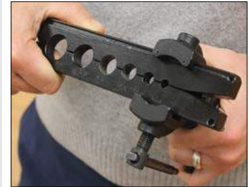
Railing allows yoke to smoothly travel while keeping the flaring tool and bar aligned
