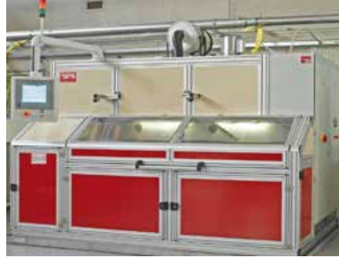
Burst test stand capable of performing burst tests on hose assemblies up to 10.000 (145000 psi)
